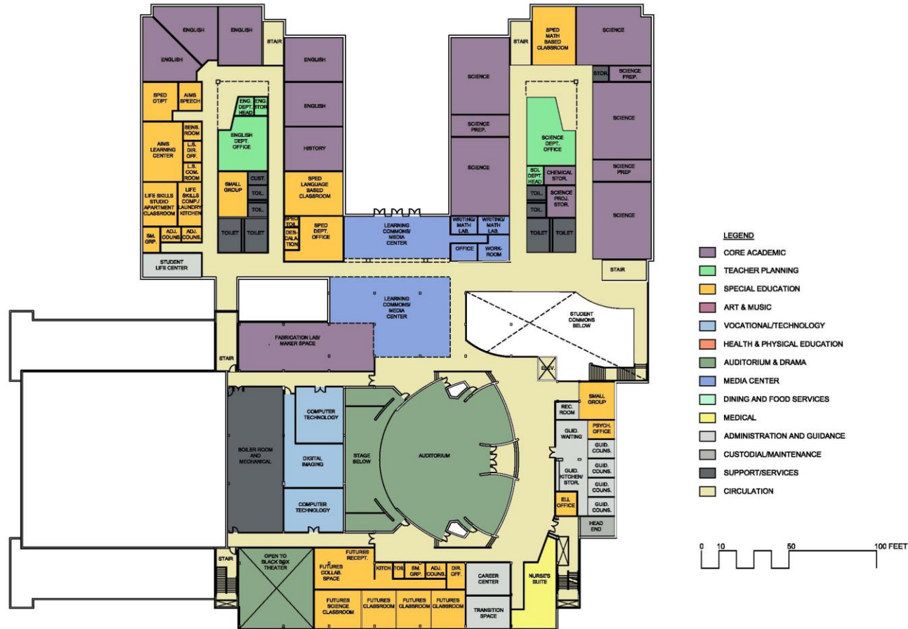
ADDITION/RENOVATION OPTION A1: MIDDLE LEVEL FLOOR PLAN
